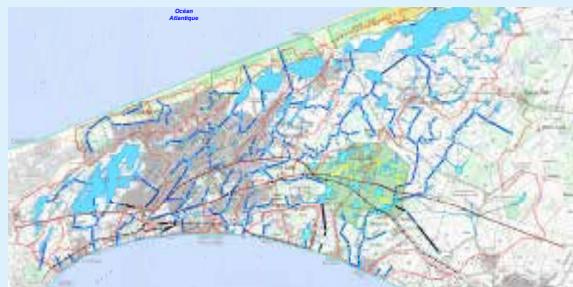
*The hydraulic diagram of the Drainage Master Plan (MDP) for stormwater in the peri-urban region of Dakar.*
